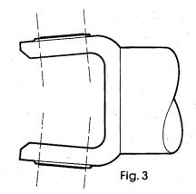
The Yoke must be properly supported when serviced (fig. 1). Any distortion of this dimension could cause difficulty in installing snap rings (fig. 2), and driveline vibration and premature bearing failure (fig. 3).
