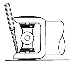
If binding is the result of yoke deformation, support the shaft and apply force as indicated. Then recheck articulation.
